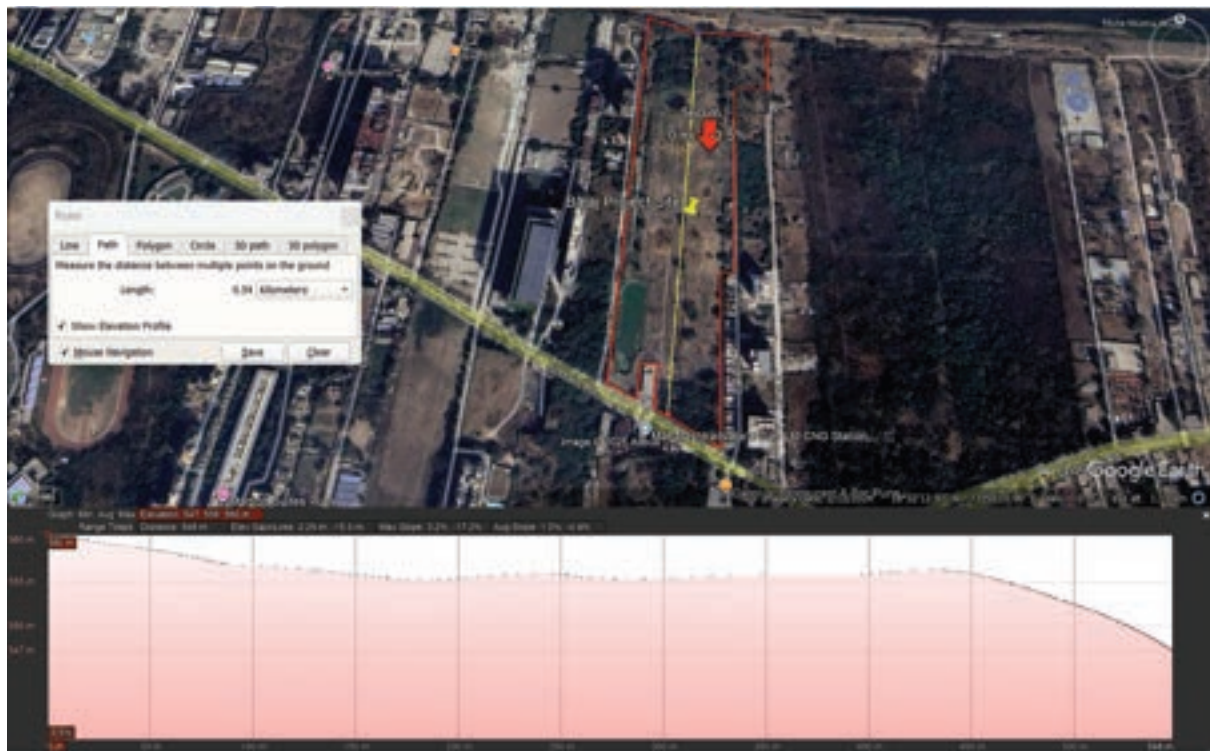
Fig 2: Elevation profile between south to north side of project site
