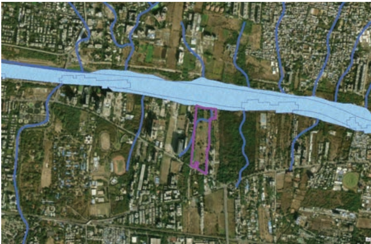
Fig 8: Drainage network map around the Project site
